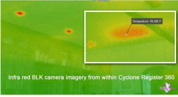
The Leica BLK360 also has a thermal camera, and when used with the Cyclone Field capture application, can reveal hotspots and spot temperature measurements can be noted visually.
